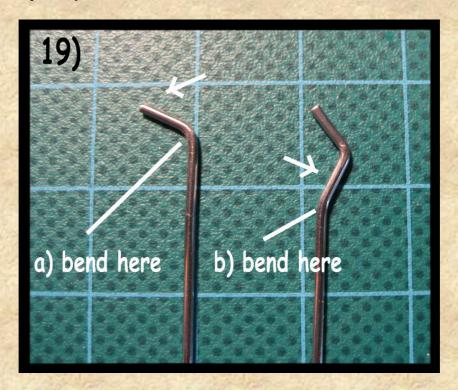
This time you can use pliers to bend the steel. Because it' not flattened and wasn't heated by now it should stand the bending. Because spring steel wire is quite strong, it took some strength to do the bending, but take your time and be careful not to hurt yourself. I found out, that the steel from the safety pin could be bent much easier this way than the conventional spring steel.
