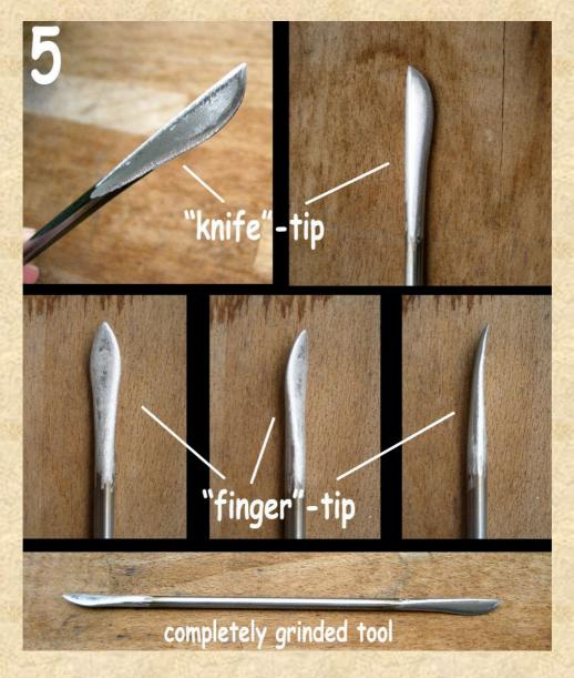
Finally I used abrasive paper and a polishing machine to remove all scratches from the tool and to give it a clean surface. In the end it looked like you can see on the next picture.
