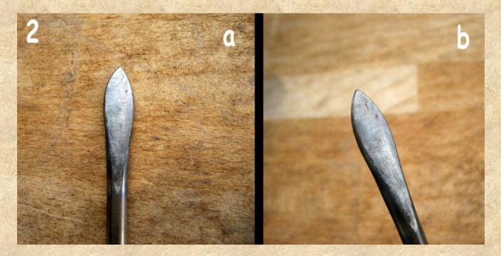
Then I moved to the other side of the stick. This end, I grinded down a bit as you can see on the next picture. The idea here is to give the end already the rough shape of the later blade of the sculpting knife. I use also the grinding machine to get this done. It's better to "pre-shape" the steel that way because it saves you a lot of work later and helps you, to get the right shape.
