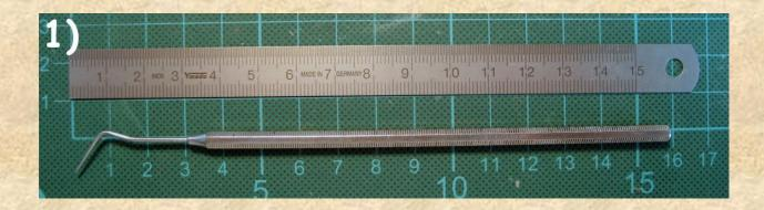
You have to cut the tip of this probe a few mm behind the first bending of the tip like you can see on pic. 2). Then you have to grind down the cut end of the tip to flatten it.
