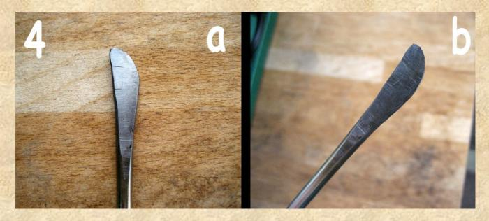
After doing the forging work, I had to refine the two ends of the tool with the grinding machine. After that, the tool looked like that:
