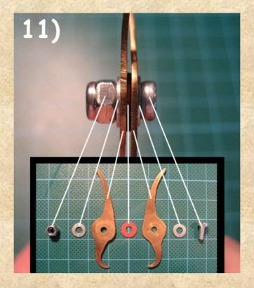
Because the ends of the two caliper claws are not exactly at the same level, you have to bent the two "claws" slightly to each other, until the points exactly meet at the same level (see pic. 12).
