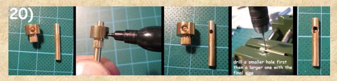
Not much more to say about that. Just place the reducing tube with the right diameter into the handle, so that the hole for the handles screw is exactly placed over the hole of the reducing tube, place a tool tip inside the reducing tube and fix it with the headless
