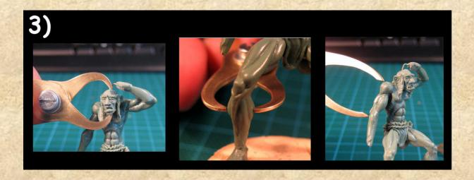
It's not difficult to build such a caliper. In short words, you just need to cut out the two "claws" of the caliper from a sheet of metal and to fix them with a bolt and nut. And that's how it goes:
