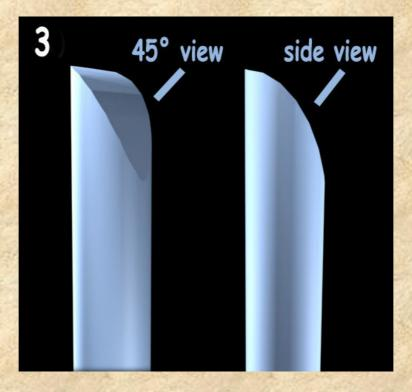
After that, this end was also flattened with heat, hammer and anvil. Again it's the same as I've explained in my post about the 1mm tool-tips for the "sculpting knife" just in a larger scale.
