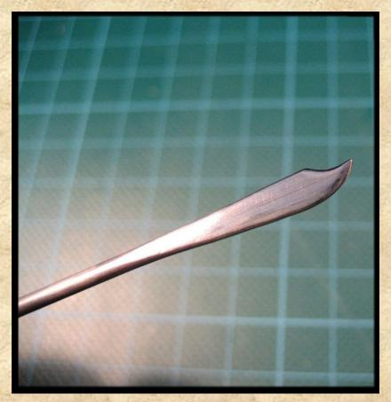
After getting the right shape, you also have to sharpen the new edge that you've created with the grinding stone.
