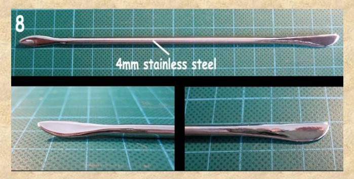
So the tools I've made by now have a diameter or "grip size" of 5mm and 4 mm. Maybe you prefer tools with a larger diameter at least at the handle. If so, here are two ways to get a thicker handle on these tools:
