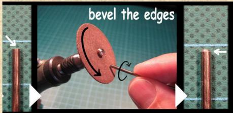
I recommend that because it makes sure, that you won't have any sharp edges left and it helps to change the tool tips in the handle because it's easier to fit the tool tip into the handle.
