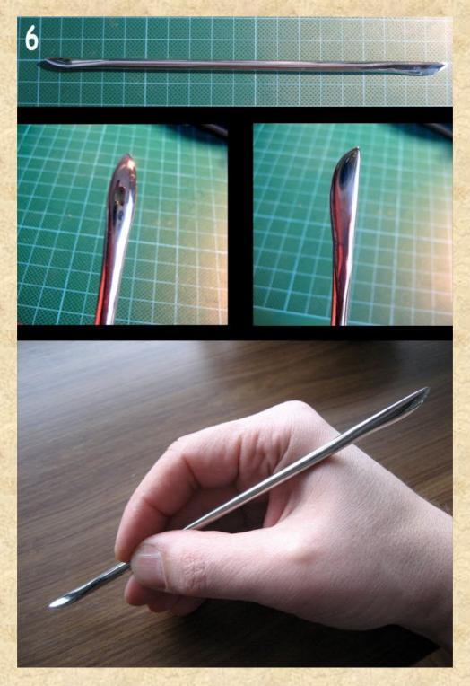
After that, the new tool was done. As I said before, it has a diameter of 5 mm, which is ok for most hands (except troll and orc).
