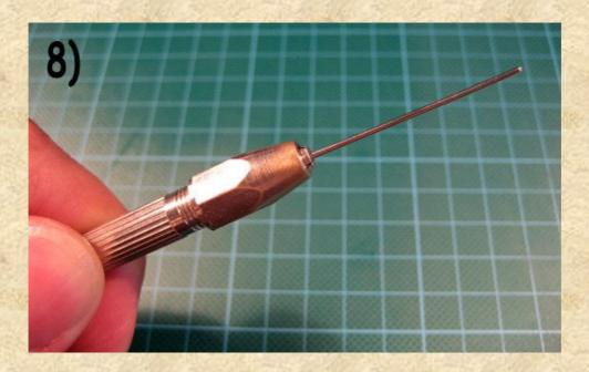
Before you start forging this steel rod, make sure, that the endpoints (were you cut the steel) are clean and flat.
