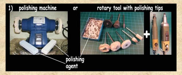
If you really want to do a lot of tool tips, maybe you should get a cheap polishing machine. That's a machine similar to the grinding-machine that I've talked about before, but just with two felt-wheels instead of the grinding stones. If you already own such a grinding machine, it's most likely, that you can buy separate felt-wheels to replace the grinding stones on your machine. That would be cheaper than buying a second machine.
