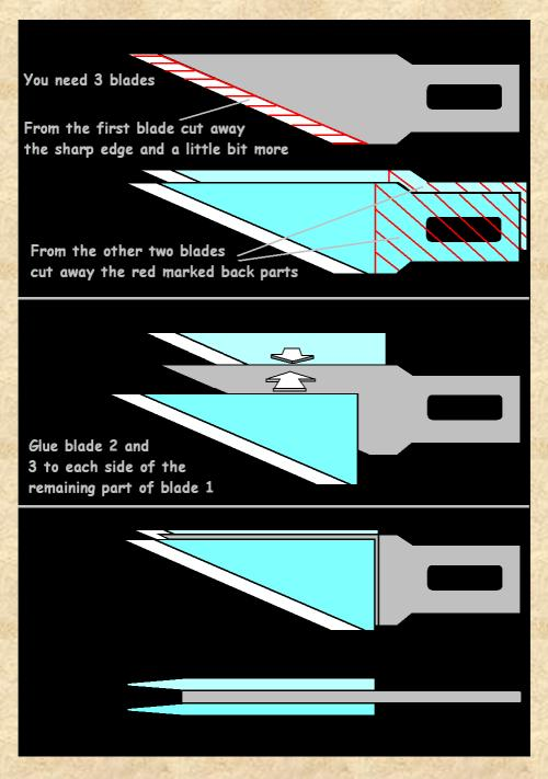
That's it. If pressed into the putty, this double blade will do belts / straps that are twice as broad as those formed by the first version of the double blade.
