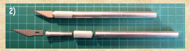
These knifes are produced in different countries and therefore the threads of the clamps of these knifes are different.
