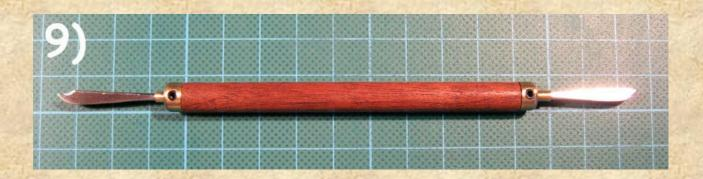
The trick about making this handle is a special kind of adjusting ring that I found via internet (pic 10.). This nice little thing is an adjusting ring made of brass with a socket to fix it into a hole.
