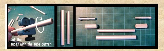
If you got your two tubes with the right length you have to clean the cut and remove all scratches from the cut edges on both tubes.
