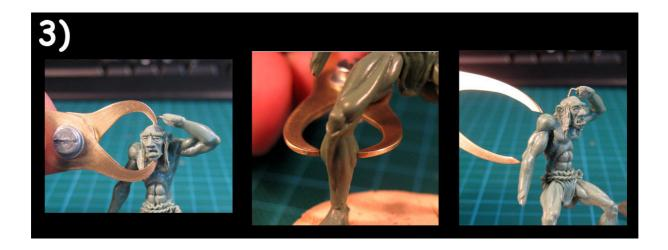
It's not difficult to build such a caliper. In short words, you just need to cut out the two "claws" of the caliper from a sheet of metal and to fix them with a bolt and nut. And that's how it goes:
