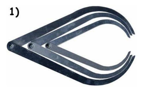
I thought, even though we do quite small sculpts, such a tool might be also useful for us miniature sculptors, so I made this miniature-version of a caliper. You can see this caliper on the next photo (pic. 2).
