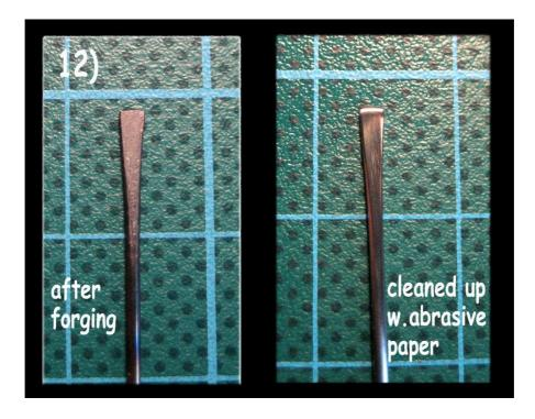
There are two alternatives for the flat sides of this spatula tool. You can leave the flat sides really "flat" with a sharper edge or you can give it a slightly round surface (see pic. 13). It's easier to get a rounded surface if you use the abrasive pads in addition to the abrasive paper. Both versions, "flat" and "rounded" have their advantages, so you should try both. Of course you can have both in one spatula: give one of the sides a flat surface and the other one a more rounded one.
