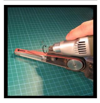
After your basic shape of the needle tip is ok, you have to give it a smooth surface by using the abrasive paper. Work from coarse grain to finer grain until the surface is free of all scratches. It's easy to achieve this by dragging the rotating steel rod (in the rotary tool) in an angle over the abrasive paper (or the abrasive pads, if you got them).
