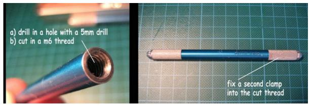
So first you have to find exact position of the centre point first. There's a trick you can: Place the handle into an electrical drilling machine (power drill) and let it rotate (not too fast). Then touch slightly the cut end of the handle with a pointed pencil. When the lead of the pencil leaves a circle, you are not in the middle, when it leaves just a point you are exactly in the middle (centre point). This point marks your centre point now and this is where you have to drill in.
