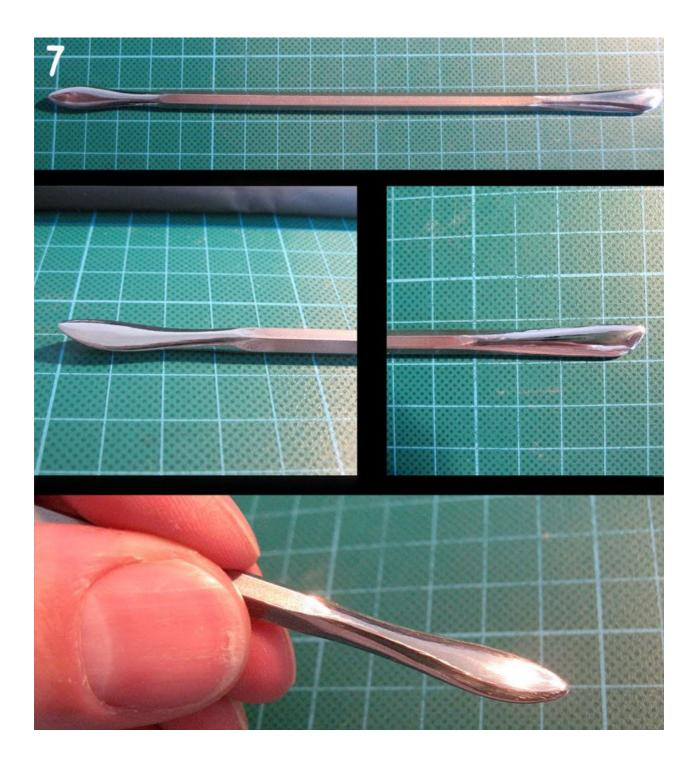
For the other alternative I used a round profile stainless steel rod again, but this time smaller with a 4 mm diameter. There's nothing special to explain here because the procedure is the same as I've explained for the first tool. This tool looks like that.
