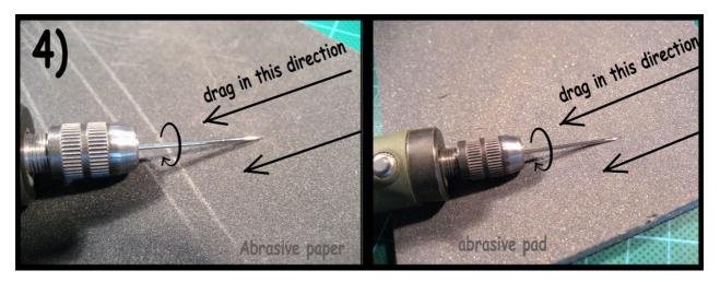
If you use the steel taken from a safety pin (See the blog entry about: Material) you are lucky, because all you have to do is to take the pointed part of the safety pin and cut off the rounded end at the right length. Just clean the cut (see above) and you are done. In most cases you don't even need to polish the needle tip taken from a safety pin, because usually it already is.
