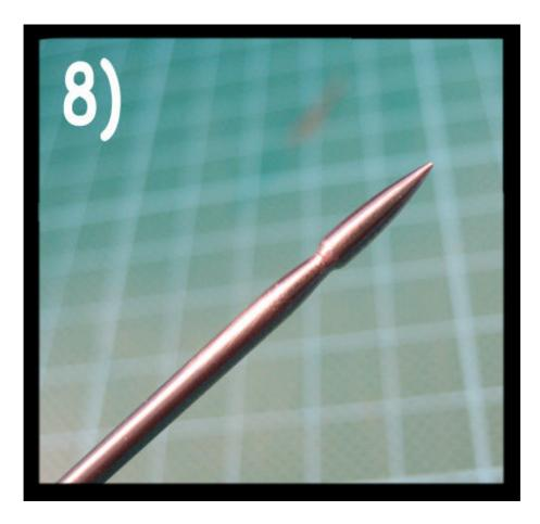
After that clean up the surface of the tool tip and remove all scratches with abrasive paper and abrasive pads (keep the steel rod rotating in the rotary tool and drag it slowly over the abrasive paper).
