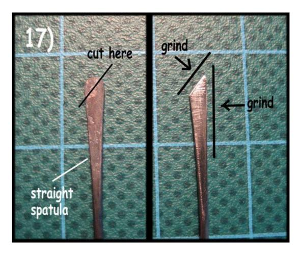
After that just make sure, to get a smooth surface on your tool tip without scratches by using the abrasive paper like I've explained before. If you are pleased with the surface, all that's left to do is to sharpen the edge of this mini knife. To do this, press the knife tip along its edge on abrasive paper with a fine grind in a 45-degree angle. Then drag it in a direction of 90-degrees to the direction of the edge, like you can see on pic. 18).
