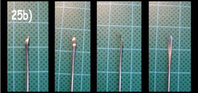
If you got the right shape it's time again for some grinding. You have to round the edges of the tool and also the flattened surface should have a slightly rounded shape. This time it is a little bit more work and it's a bit more difficult, because of the form of the tool tip and because the edges should be much rounder as on the spatula tool tips for example. Once again an abrasive pad would make this job easier.
