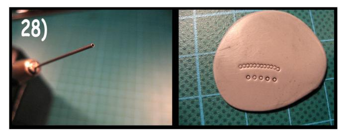
As I said, with this tool, you can create a rivet like structure while pressing the end of the tube into the putty like you see on pic. 28. So basically it's the simplest form of a "stamptool". In a later tutorial I will tell you a little bit more about the use of stamp tools for sculpting miniatures.
