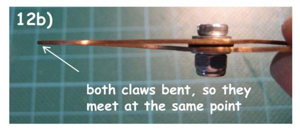
Screw the nut and bolt as tight that there is some resistance while opening and closing the calipers claws while they can still be moved smoothly.
