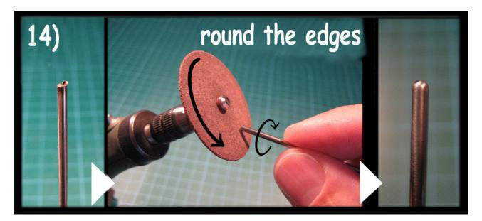
Again, it's quite easy to achieve this rounded end with the rotary tool and the cutting wheel. Be sure to rotate the rod slightly between your fingers while holding it onto the cutting wheel. You could also use just abrasive paper for that, but it's much more work and it's harder to achieve a "clean" rounded shape.
