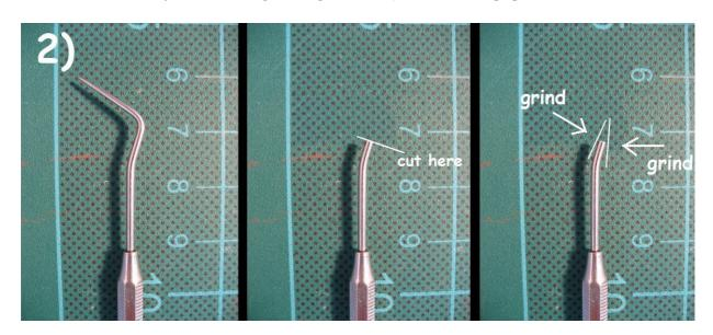
Just give it a smooth surface and round off all edges. Finally the tip should look like those you can see on pic. 3) and pic. 4). Be sure to give it a clean surface with no scratches left.
