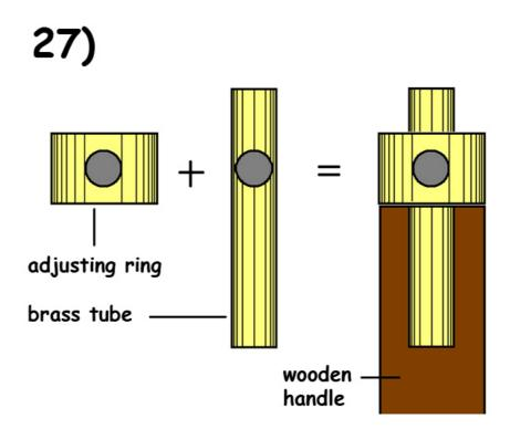
For doing that you have to find ordinary adjusting rings with the right size. As I prefer sculpting handles with a diameter of 8 mm, the adjusting rings should also have an outer diameter of 8mm. The inner diameter depends on the size of the sculpting tool tips, you want to fix in the handle later.
