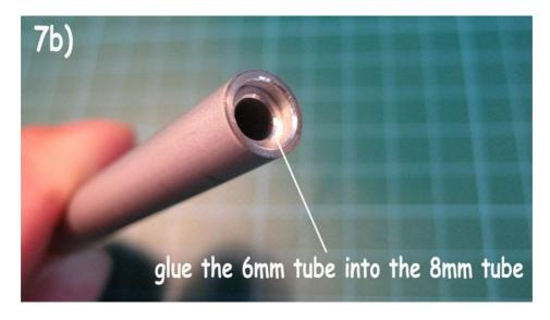
Now give the glue some time to get hard. Be sure, that the glue is completely hardened before going on. I recommend waiting for two days before going on.
