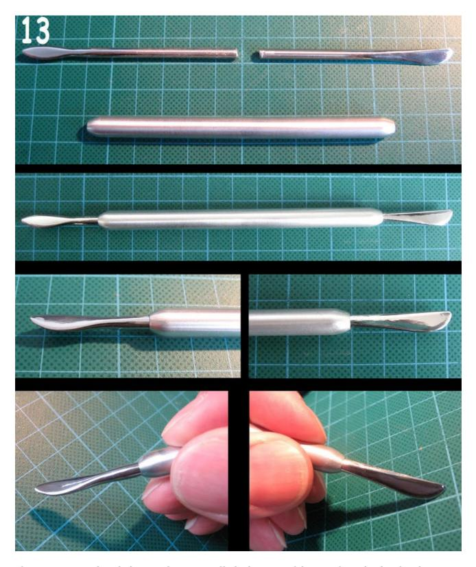
If you want to make a lighter tool, just cut off a little more of the non-forged side of each tool tip before gluing it into the aluminium handle.
