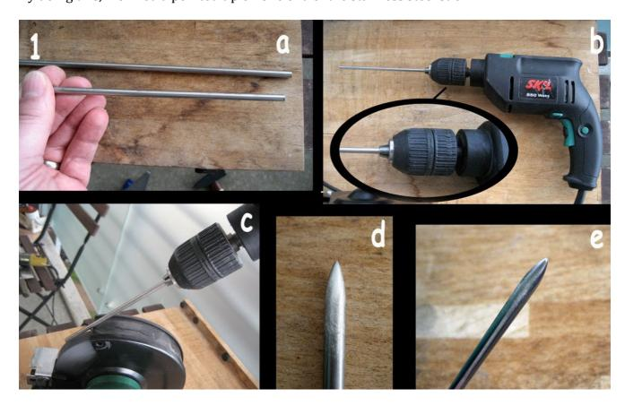
After that, I just flattened the end of the stick. To do so, I heated the pointed end of the stick up until it glows and than hammered it down on an anvil. It's just the same
