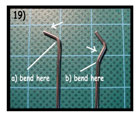
This time you can use pliers to bend the steel. Because it' not flattened and wasn't heated by now it should stand the bending. Because spring steel wire is quite strong, it took some strength to do the bending, but take your time and be careful not to hurt yourself. I found out, that the steel from the safety pin could be bent much easier this way than the conventional spring steel.
