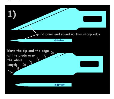
Just refine the edges and the surface of the grinded blade with very fine abrasive paper or abrasive pads. You can finally polish it, if you like.
