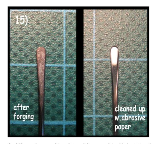
You see the difference between this tool tip and the one explained before is just the rounded edge at the top instead of the straight edge on the tool tip before. This difference may look small, but while sculpting it makes a big difference.
