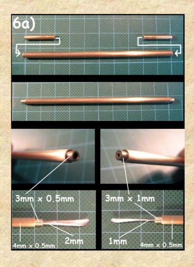
You can also make a handle with 6 mm diameter with a combination of aluminium and brass tubes that have to be glued together like you can see on pic. 6b).
