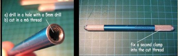
So first you have to find exact position of the centre point first. There's a trick you can: Place the handle into an electrical drilling machine (power drill) and let it rotate (not too fast). Then touch slightly the cut end of the handle with a pointed pencil. When the lead of the pencil leaves a circle, you are not in the middle, when it leaves just a point you are exactly in the middle (centre point). This point marks your centre point now and this is where you have to drill in.
