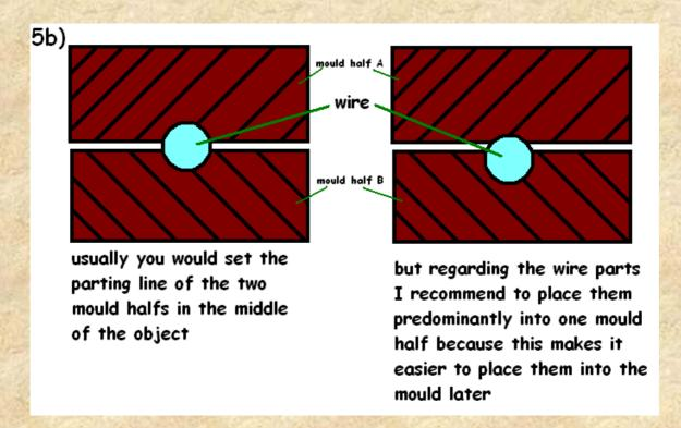
When you've got your mould with cut in gate, sprues and air vents you can try your first cast. Before you cast the white metal into your mould, you have to place two bent pieces of wire inside the mould as you can see on pic. 6a and 6b).
