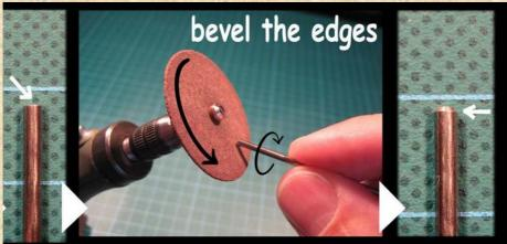
I recommend that because it makes sure, that you won't have any sharp edges left and it helps to change the tool tips in the handle because it's easier to fit the tool tip into the handle.
