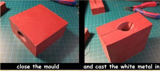
First you have to straighten the two pieces of wire. Then you have to bend them at the right point into the needed angle with a flat nose plier. You have to try a little bit to get the right angle. Place the wire parts into one half of the mould at the right position. Then carefully close the mould without letting the wire parts slip out of their positions.
