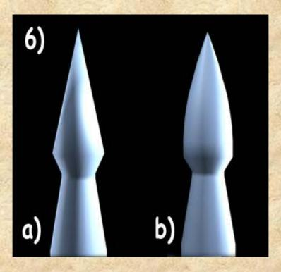
Then cut in a circular furrow under the tip. Don't make this furrow too deep but just enough to form the cone-like tip. You'll have to bend the steel later.
