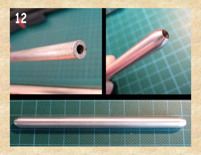
After that, I just cut the forged tool in the middle and glued each part into one end of the aluminium too with good metal glue.
