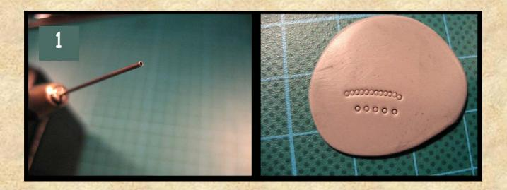
Basically a stamp tool is an object with some kind of structured or engraved surface. If you press it on or into your putty, it leaves a mirrored-inverted mark on the putty. By using stamp tools, you can save a lot of time and you can do details that are nearly impossible to achieve by trying to do them by hand (unless you are Tom Meier).
