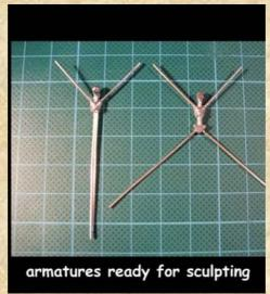
If your armature didn't come out right from the mould, it's maybe because the mould is too cold in the beginning, so just try again. After some casts, the mould should get its working temperature. If the results are still not good, try to widen the cut, where the gate "touches" the cavity and/or cut some additional air vents.
