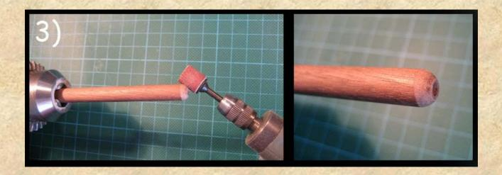
If you got a nicely bevelled handle, you have to give it a good surface by using fine abrasive paper.
