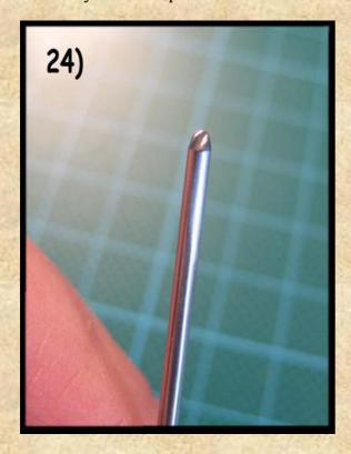
When you got this, start flatten the end of the steel wire with hammer and anvil after heating it up, like I explained above.
