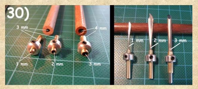
So just glue this part into the hole in the handle as I've explained above. As before, you can use handles made of wood or aluminium.
