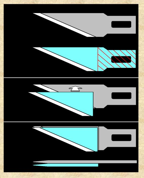
You can place the finished double blade into the handle of the hobby-knife, like any other blade. That's the reason, why you have to cut away the back part of one of the blades, because two blades wouldn't fit into the handle at the same time. At least that's the case with my hobby-knife handles. If you got a handle that can hold two parallel blades at the same time, you don't have to cut away anything, just glue two blades together and you are done.
