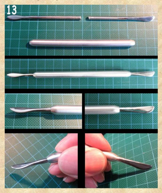
If you want to make a lighter tool, just cut off a little more of the non-forged side of each tool tip before gluing it into the aluminium handle.
