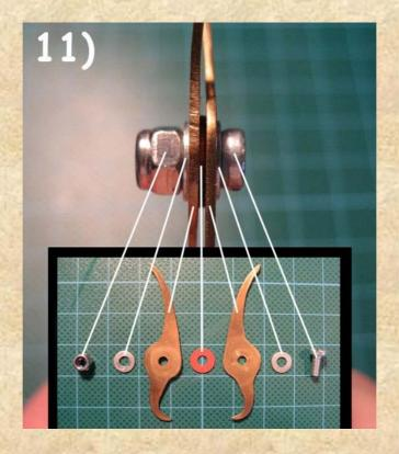
Because the ends of the two caliper claws are not exactly at the same level, you have to bent the two "claws" slightly to each other, until the points exactly meet at the same level (see pic. 12).
