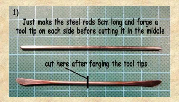
Another thing that belongs to all tool tips, regardless if made of 1mm, 1,5mm, 2mm, or 3mm is how to treat the back-side of the tool tips, I mean the side that fits into the handle. I recommend, to
