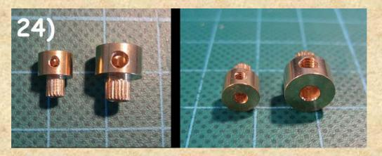
As the inner diameter of the 6mm aluminium tool is 4mm, you have to use short pieces of a brass tube (with outer diameter: 4mm / inner diameter: 3mm / material strength: 0.5 mm) in a similar way as I described for version 2) above.
