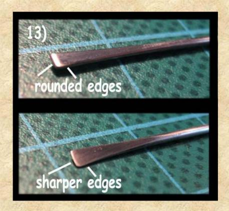
All that's left now is to cut your tool tip to the right length, refine the cut end like explained above and polish your tool tip (more about polishing later). Ta-dah... Your first forged tool tip is done.
