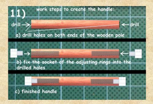
Now the little tool, I've talked about before, comes into play. I've combined an aluminium tube and a brass tube to form a drilling-aid. With this aid, you can place and keep the drill exactly in the centre point of the tool handle while drilling.
