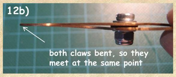
Screw the nut and bolt as tight that there is some resistance while opening and closing the calipers claws while they can still be moved smoothly.
