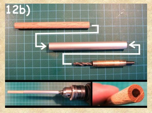
Obviously, the final hole has to be as deep (or a little deeper to stay flexible) as the tool tip will stuck into it.
