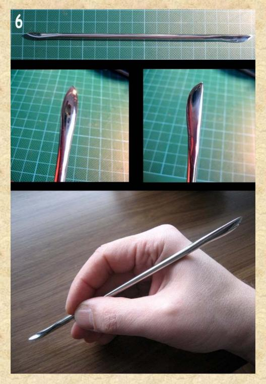
After that, the new tool was done. As I said before, it has a diameter of 5 mm, which is ok for most hands (except troll and orc).
