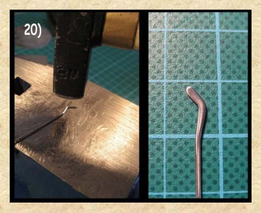
Again remove all scratches from the tool tips surface with the abrasive paper and you're done.
