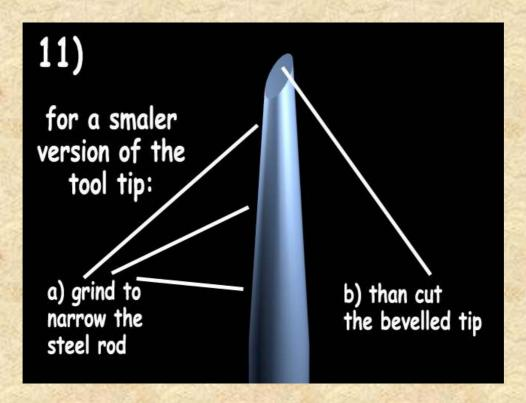
Then you have to clean the surface from the scratches as always. But be sure to leave the edges at the narrowed tip "sharp".
