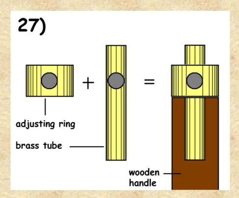
For doing that you have to find ordinary adjusting rings with the right size. As I prefer sculpting handles with a diameter of 8 mm, the adjusting rings should also have an outer diameter of 8mm. The inner diameter depends on the size of the sculpting tool tips, you want to fix in the handle later.
