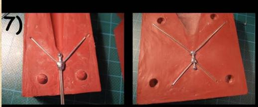
Cast armatures in the mould (on the pictures, the sprue is already removed)
