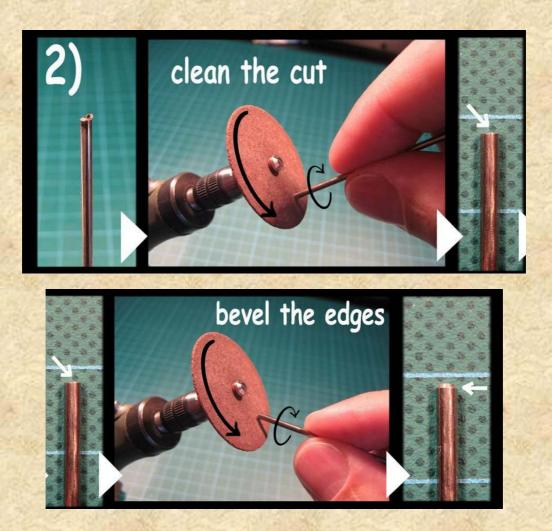
I recommend that because it makes sure, that you won't have any sharp edges left and it helps to change the tool tips in the handle because it's easier to fit the tool tip into the handle.
