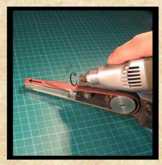
After your basic shape of the needle tip is ok, you have to give it a smooth surface by using the abrasive paper. Work from coarse grain to finer grain until the surface is free of all scratches. It's easy to achieve this by dragging the rotating steel rod (in the rotary tool) in an angle over the abrasive paper (or the abrasive pads, if you got them).
