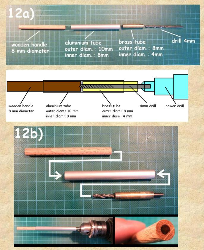
Obviously, the final hole has to be as deep (or a little deeper to stay flexible) as the tool tip will stuck into it.
