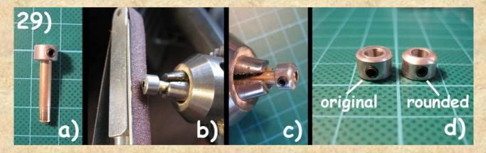
If you've done this, just glue the brass tube into the hole of the adjusting ring so the headless screw can go through the hole in the brass tubes side.
