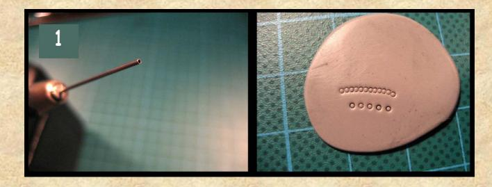
Basically a stamp tool is an object with some kind of structured or engraved surface. If you press it on or into your putty, it leaves a mirrored-inverted mark on the putty. By using stamp tools, you can save a lot of time and you can do details that are nearly impossible to achieve by trying to do them by hand (unless you are Tom Meier).
