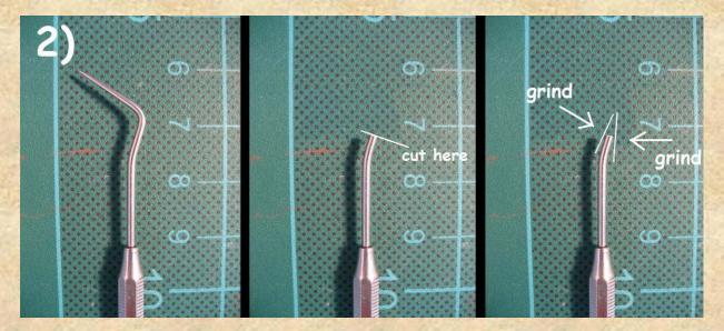
Just give it a smooth surface and round off all edges. Finally the tip should look like those you can see on pic. 3) and pic. 4). Be sure to give it a clean surface with no scratches left.
