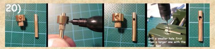
Not much more to say about that. Just place the reducing tube with the right diameter into the handle, so that the hole for the handles screw is exactly placed over the hole of the reducing tube, place a tool tip inside the reducing tube and fix it with the headless
