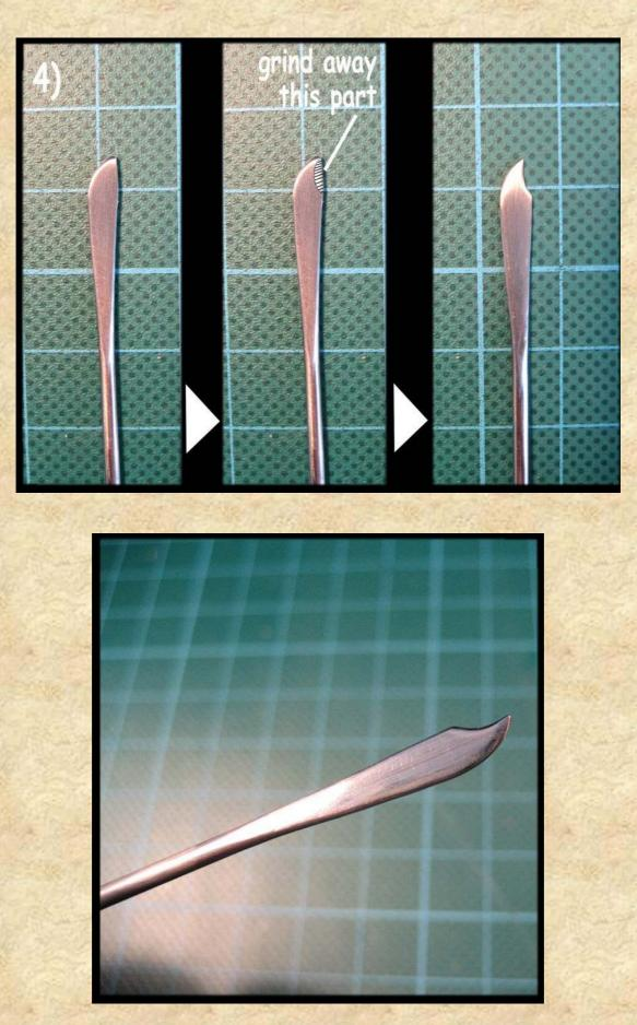
After getting the right shape, you also have to sharpen the new edge that you've created with the grinding stone.
