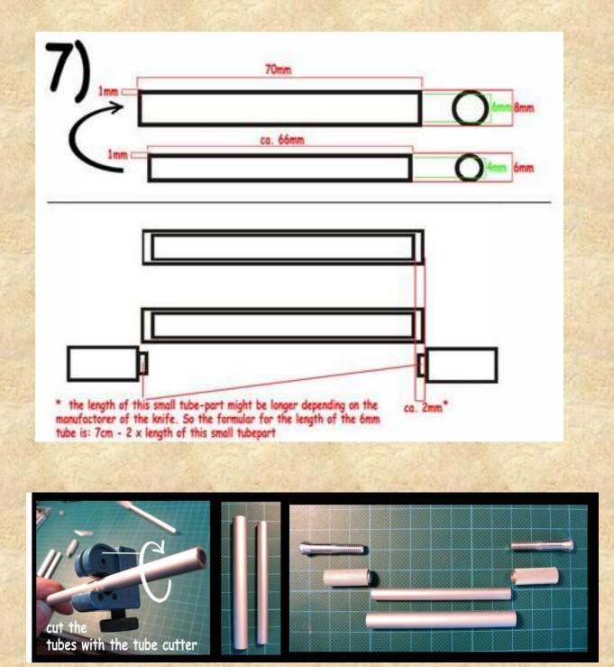
If you got your two tubes with the right length you have to clean the cut and remove all scratches from the cut edges on both tubes.
