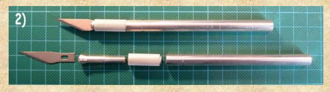
These knifes are produced in different countries and therefore the threads of the clamps of these knifes are different.
