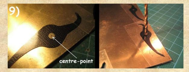
The reason for me to recommend drilling before cutting out the rest is that the "cutting out" is quite a bit of work. So if you would do the cutting first and the later drilling went wrong, all the cutting-work with the saw will be lost. So I guess it's better to start with the holes.
