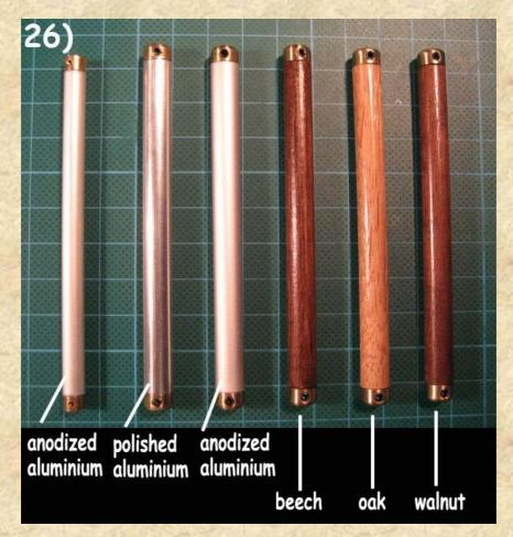
So, that's nearly all about the handles, I've developed for holding the tool tips.
