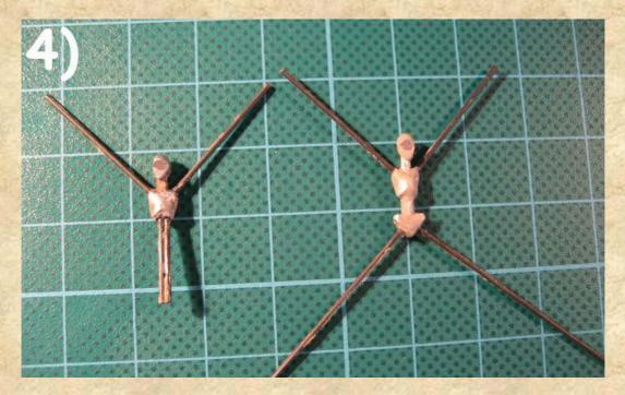
To fix the wire parts, I just drill in small holes into the sculpted part and glued the wire in. I used wire with a diameter of 0.8 mm for that.
