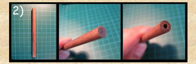
A surprisingly difficult part is to drill the hole into the wooden handle exactly centred and straight. Maybe you should drill in a guiding hole with a smaller drill first.
