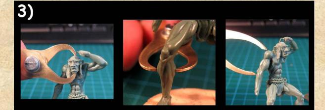
It's not difficult to build such a caliper. In short words, you just need to cut out the two "claws" of the caliper from a sheet of metal and to fix them with a bolt and nut. And that's how it goes:
