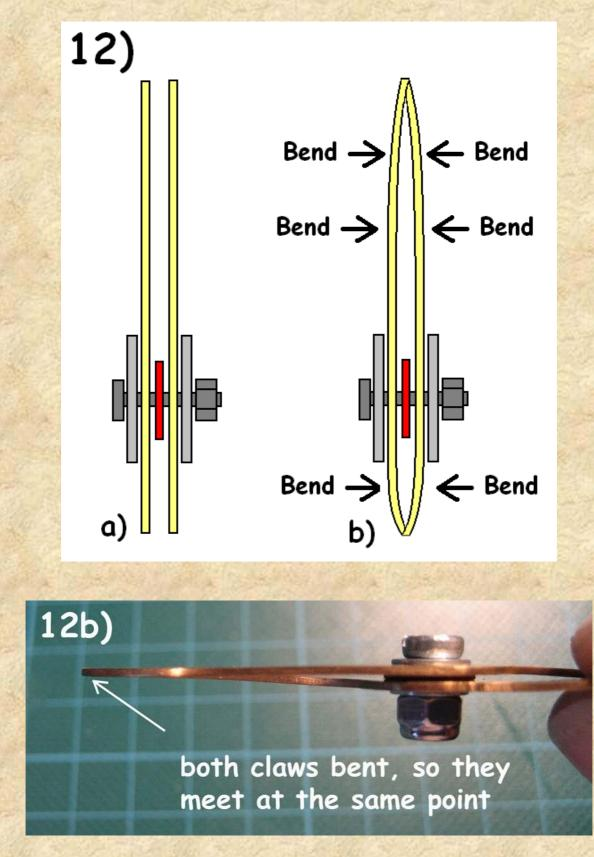
Screw the nut and bolt as tight that there is some resistance while opening and closing the calipers claws while they can still be moved smoothly.
