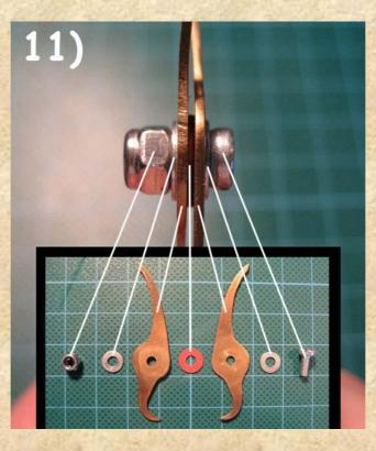
Because the ends of the two caliper claws are not exactly at the same level, you have to bent the two "claws" slightly to each other, until the points exactly meet at the same level (see pic. 12).
