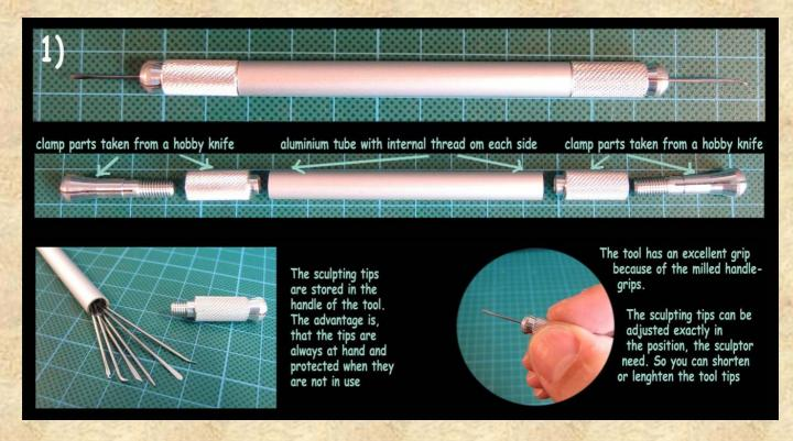
If you ask yourself why I wrote in the title of this post "the hard way", it's because you have to do a little metal working like cutting threads for example. There is also an "easy way" to get a kind of a Schellert Tool which is nearly as good as the original one with a minimum of work. I'll tell you in a later tutorial how to do this.
