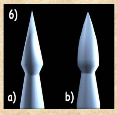
Then cut in a circular furrow under the tip. Don't make this furrow too deep but just enough to form the cone-like tip. You'll have to bend the steel later.
