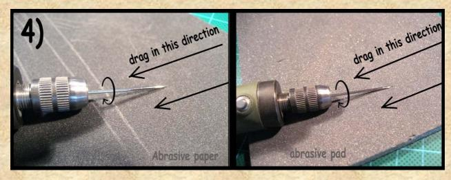
If you use the steel taken from a safety pin (See the blog entry about: Material) you are lucky, because all you have to do is to take the pointed part of the safety pin and cut off the rounded end at the right length. Just clean the cut (see above) and you are done. In most cases you don't even need to polish the needle tip taken from a safety pin, because usually it already is.
