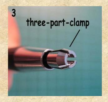
So just file or grind down the back end of your tool tip, until it gets a slightly triangular shape (pic. 4). In most cases, that should solve the "rotating-problem", but I have to admit, that this rotating thing is a weak point of the pencil tools.
