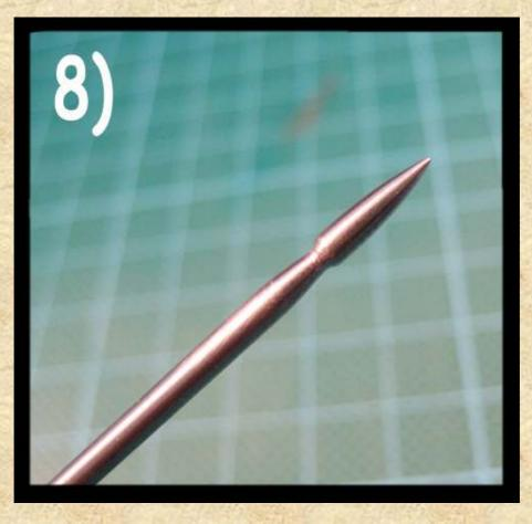
After that clean up the surface of the tool tip and remove all scratches with abrasive paper and abrasive pads (keep the steel rod rotating in the rotary tool and drag it slowly over the abrasive paper).
