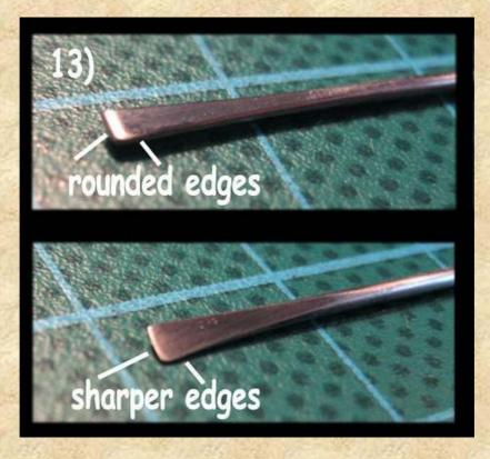
All that's left now is to cut your tool tip to the right length, refine the cut end like explained above and polish your tool tip (more about polishing later). Ta-dah... Your first forged tool tip is done.
