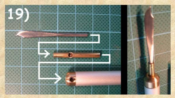
To drill in the hole into the sides of the tubes, just fit them into the handle (adjusting ring).
