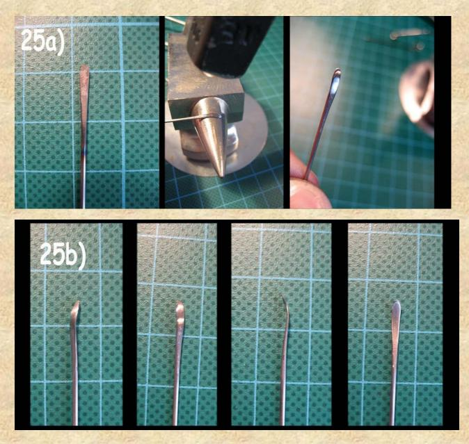
If you got the right shape it's time again for some grinding. You have to round the edges of the tool and also the flattened surface should have a slightly rounded shape. This time it is a little bit more work and it's a bit more difficult, because of the form of the tool tip and because the edges should be much rounder as on the spatula tool tips for example. Once again an abrasive pad would make this job easier.
