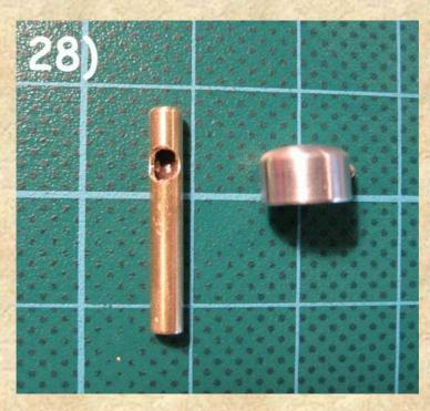
You can round (bevel) the upper edge of the adjusting ring just like I've explained before for the "special adjusting rings with socket (on pic. 28) above, the ring has already been rounded).
