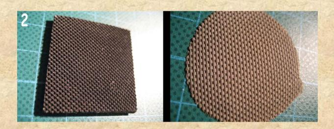
Other interesting structures could be achieved by using for example rough sandpaper (abrasive paper) that is pressed onto the putty.
