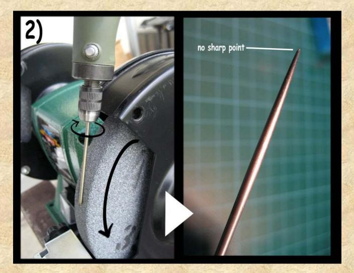
After grinding down the wire rod to the right shape, as always, you have to smooth the surface and remove all scratches.
