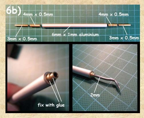
Finally glue in a tooltip in the hole of each insert-tube.
