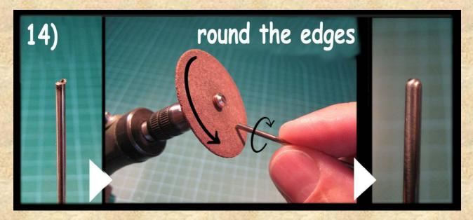
Again, it's quite easy to achieve this rounded end with the rotary tool and the cutting wheel. Be sure to rotate the rod slightly between your fingers while holding it onto the cutting wheel. You could also use just abrasive paper for that, but it's much more work and it's harder to achieve a "clean" rounded shape.
