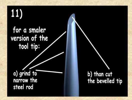
Then you have to clean the surface from the scratches as always. But be sure to leave the edges at the narrowed tip "sharp".
